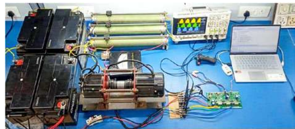
Controller Circuit Board Developed for E-Rickshaw and Tested for Field Applications
